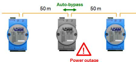
Furthermore, for the reason of signal transmission characteristics, the continuous auto-bypass node should be less than 2, so that the network communication in daisy chain wiring is workable.
