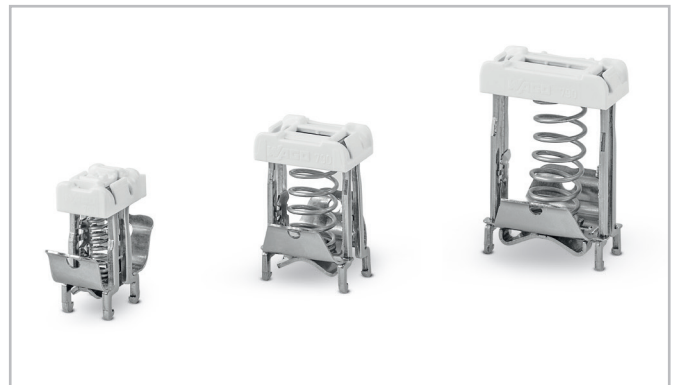
WAGO's next generation of shield clamping saddles – with their patented latching mechanism for force-free mounting.
