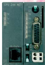
TCP/IP PLC-CPU 241-244NET with Ethernet-CP
