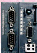
PLC-CPU 214-216SER with 2 RS232C-serial interfaces
