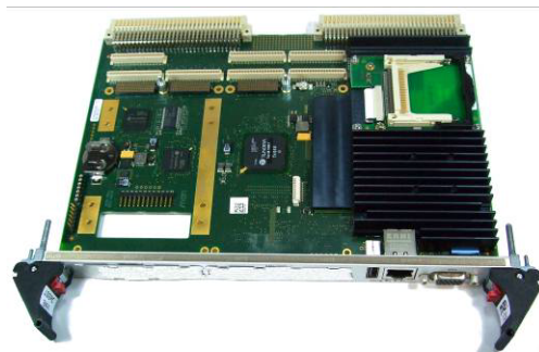
Fig. 1: VMEbus PC with Intel Core architecture and XMC/PMC slots (MEN A20)
