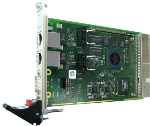
Fig.2: CompactPCI slave CPU with e300 PowerPC (MEN F218)
