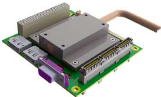
Figure 1: Heat pipe cooling system using heat spreader
