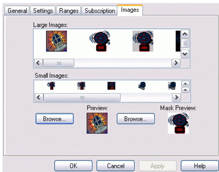
AlarmWorX32 Indicator ActiveX Control Properties: Images Tab
