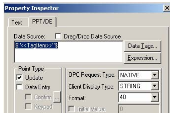
Figure 2 - Process Point Property Inspector
