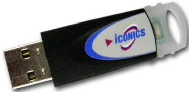
Figure 1 – Sentinel-style ICONICS USB hardware key
