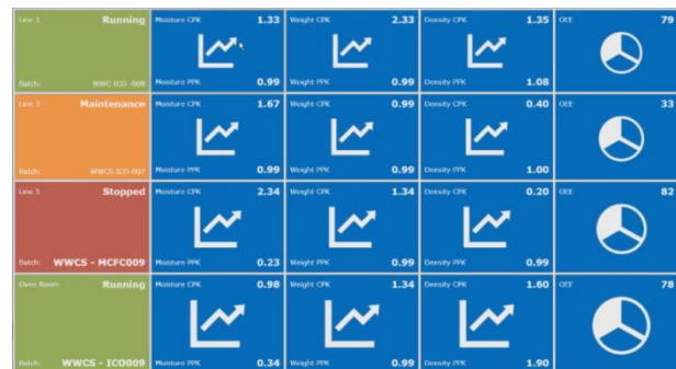
Figure 8 - Using SPC data in Smart Tiles
