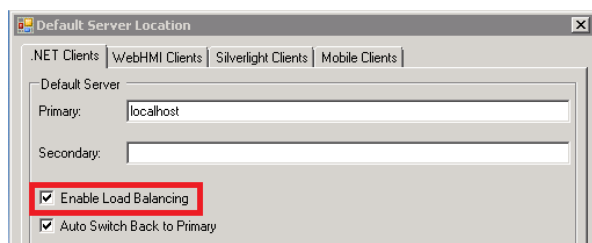
Figure 4 - Configuration for Load Balancing servers
