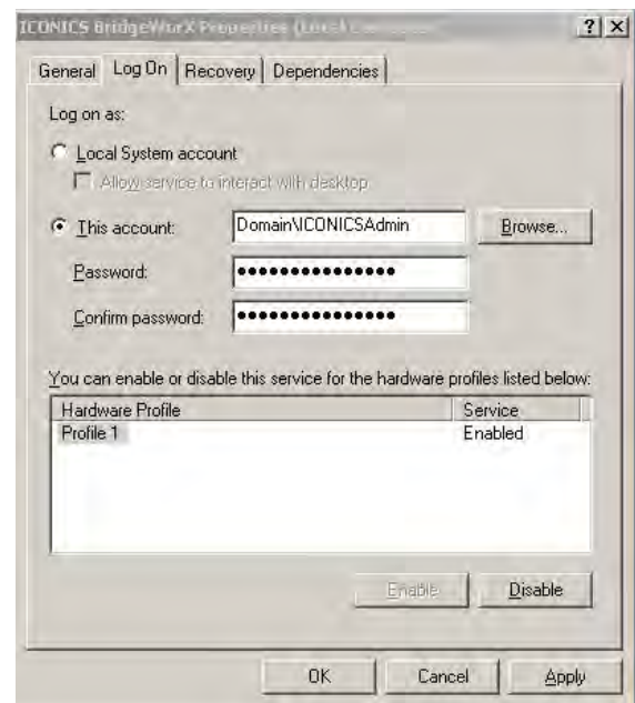
Figure 5 – BridgeWorX NT Service – Log On
