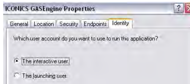
Figure 6 - DCOM Properties Identity Tab
