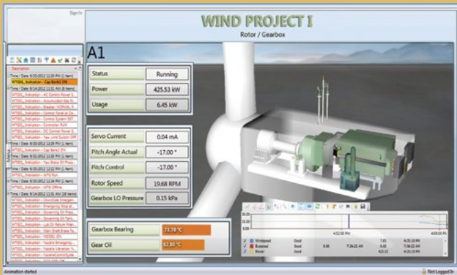
An AES Turbine Screen, Built with GENESIS64
