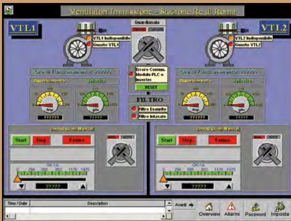
Ventilation Monitoring and Control for Rome Metro S.p.A.
