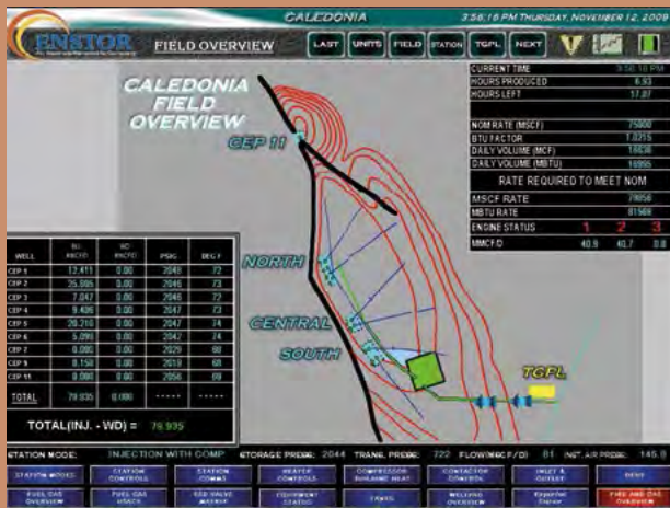
Overview of the Caledonia Storage Facility
