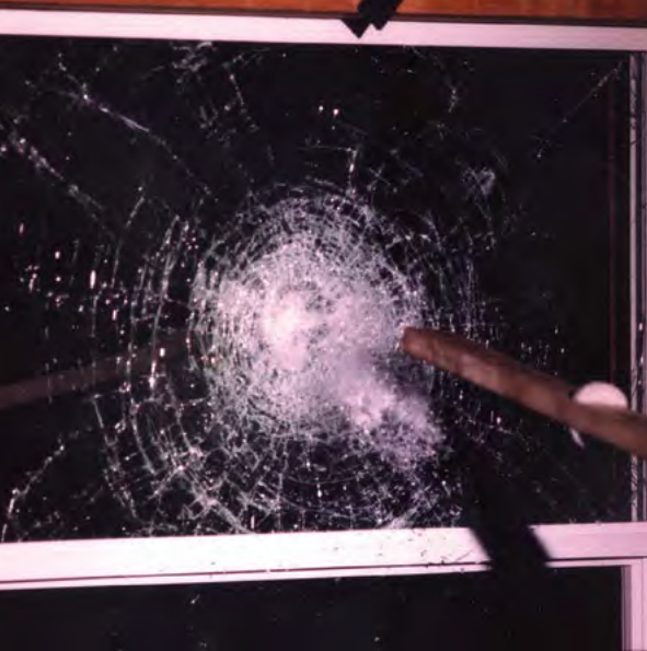
Glass Impact Testing at PGT's North Venice Production Facility
