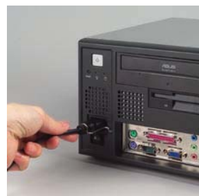
Plug ring-lock securely fastens the power cord
