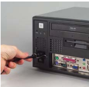
Plug ring-lock securely fastens the power cord
