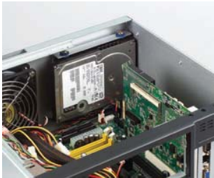
Shock-resistant drive bay for holding an internal 3.5" HDD
