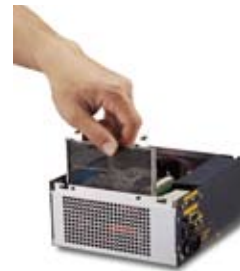
Hot swappable filter for easy replacement
