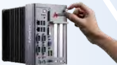
1. Undo the thumbscrew by hand
