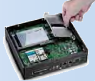
3. Flexible memory expansion slots
